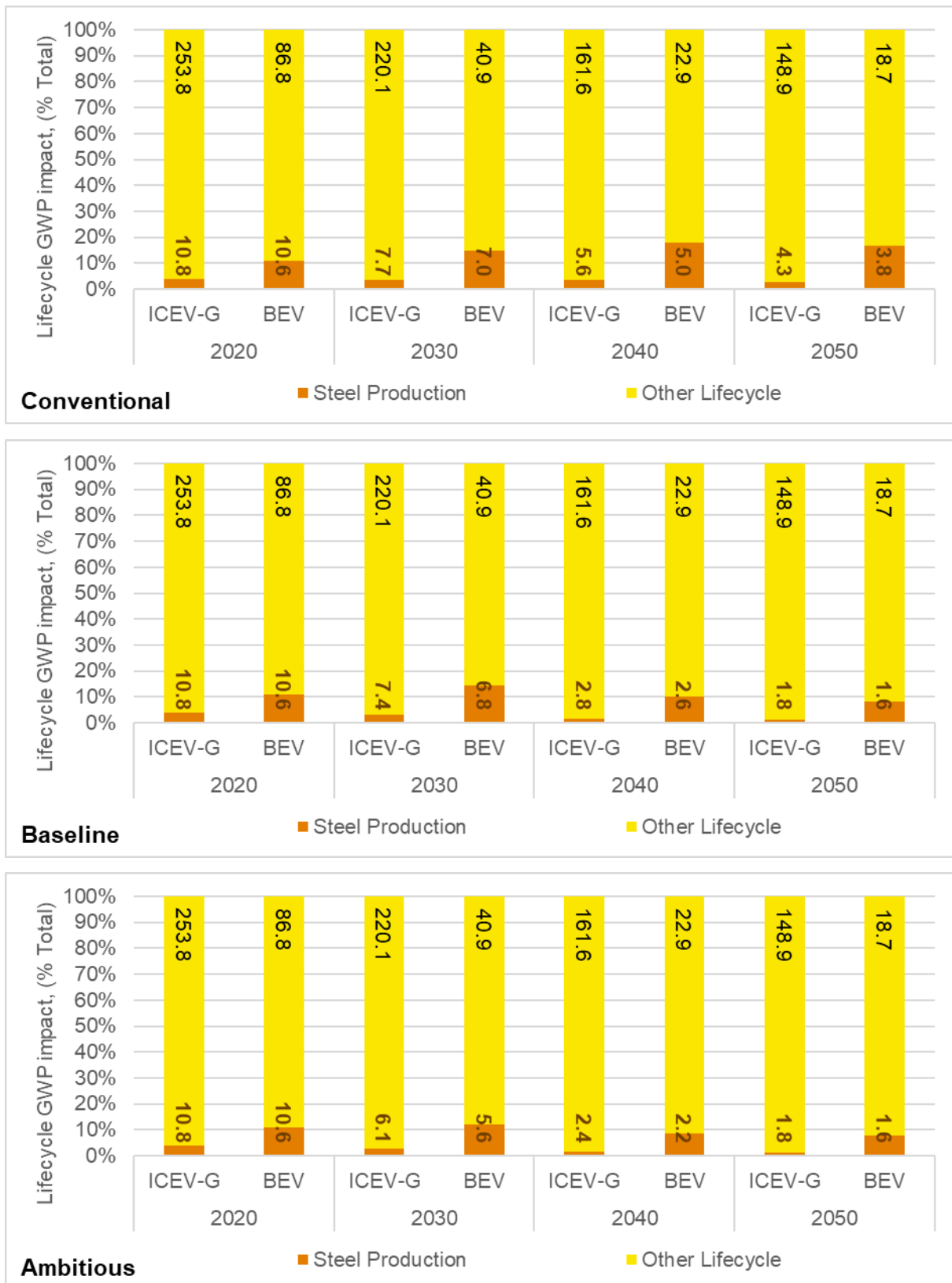
Figure A6: Share of steel production emissions of total passenger car lifecycle emissions, 2020-2050, for Conventional, Baseline and Ambitious Scenario pathways. In-graph absolute values are in gCO 2 e/vkm.
