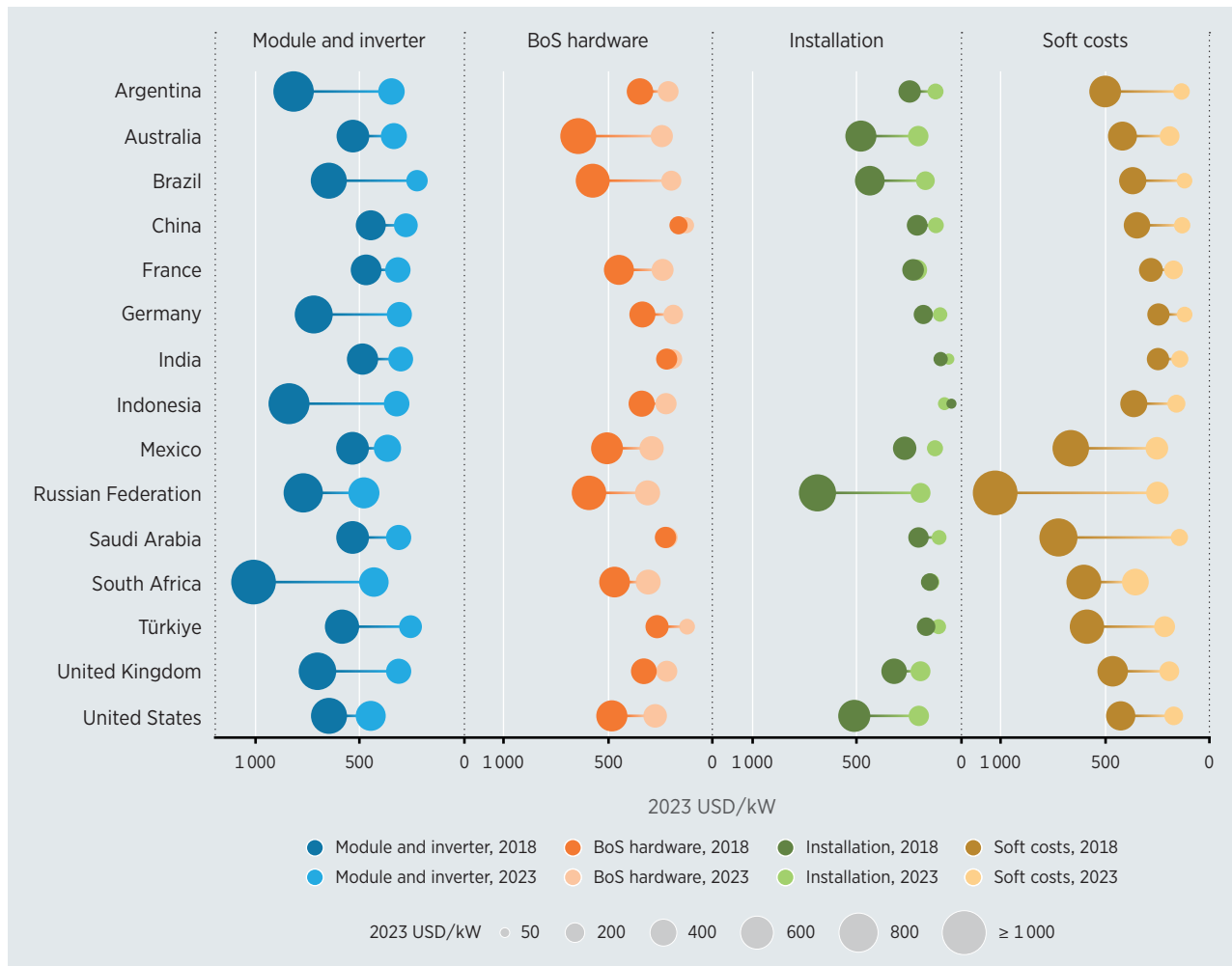
Figure 3.7 Breakdown of utility-scale solar PV total installed costs by country, 2018 and 2023
