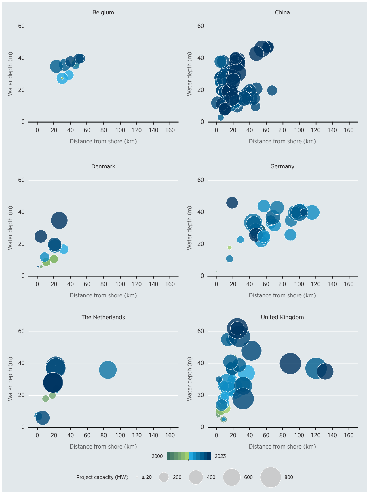
Figure 4.3 Distance from shore and water depth for offshore wind projects by country, 2000-2023
