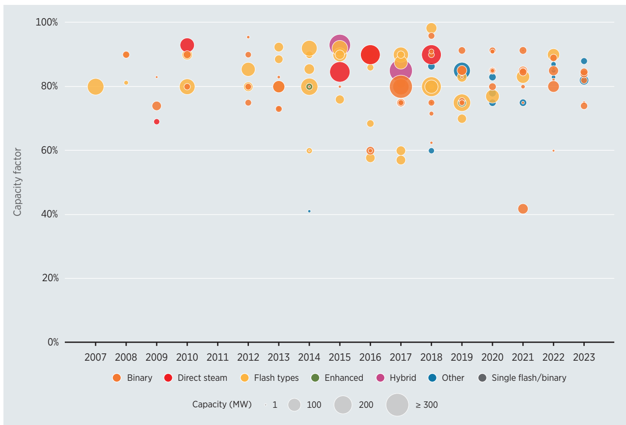
Figure 8.3 Capacity factors of geothermal power plants by technology and project size, 2007-2023
