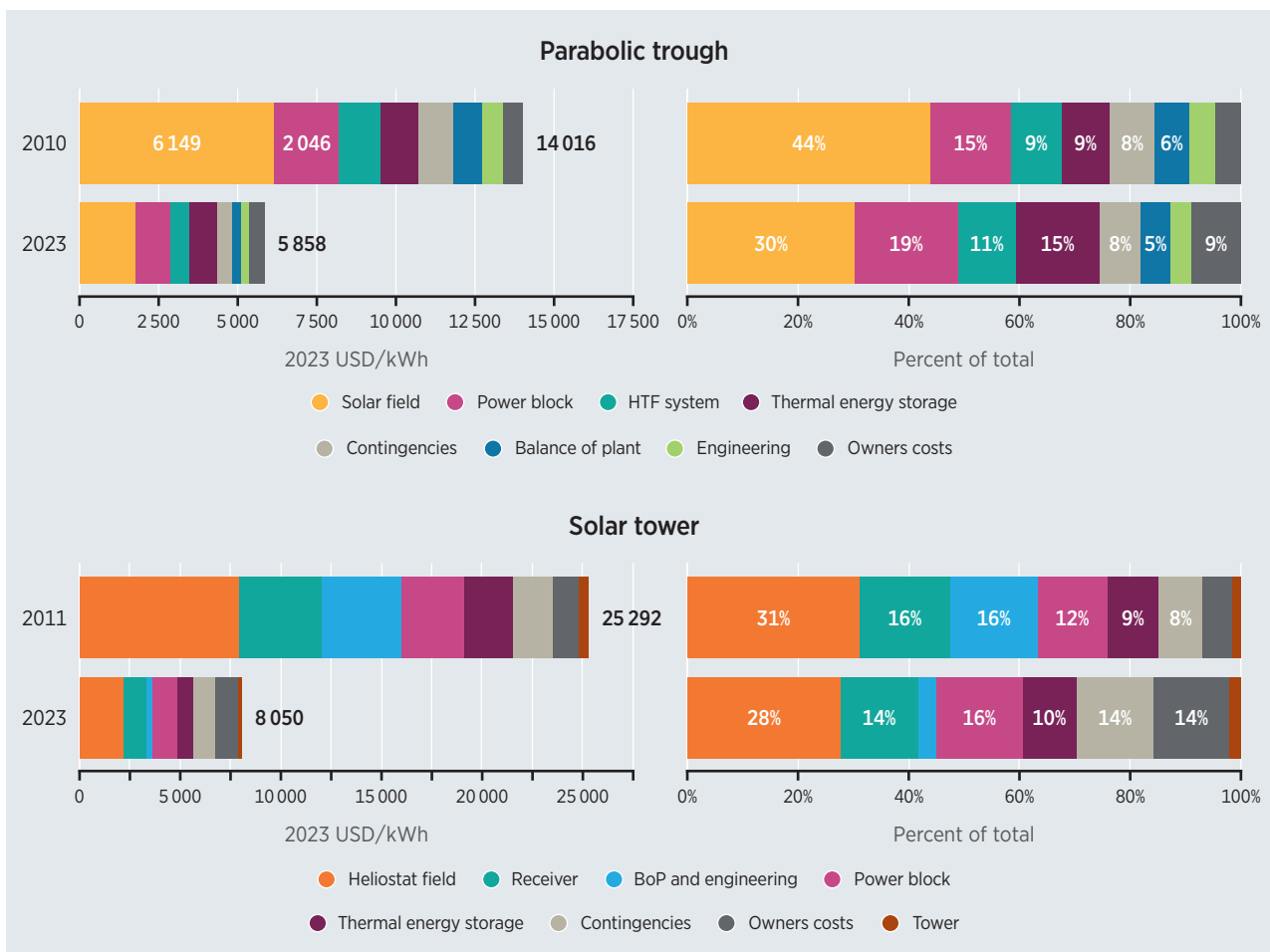
Figure 5.3 Total installed cost breakdown of CSP plants by technology, 2010-2011 and 2023
