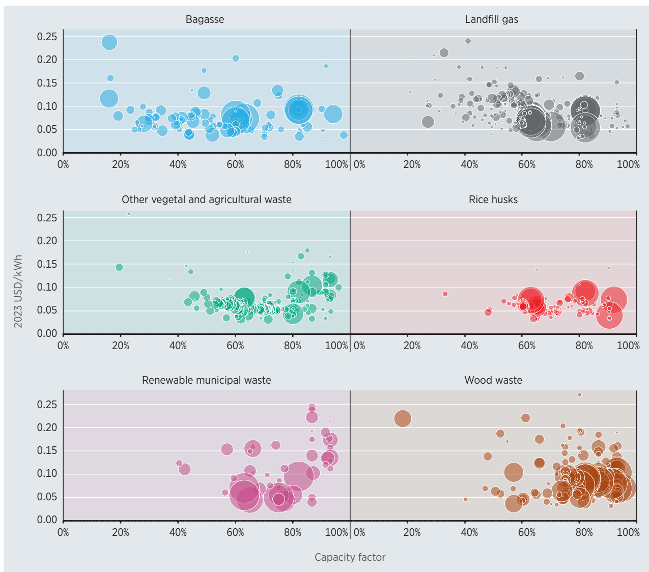
Figure 9.6 LCOE and capacity factor by project of selected feedstocks for bioenergy power generation projects, 2000-2023
