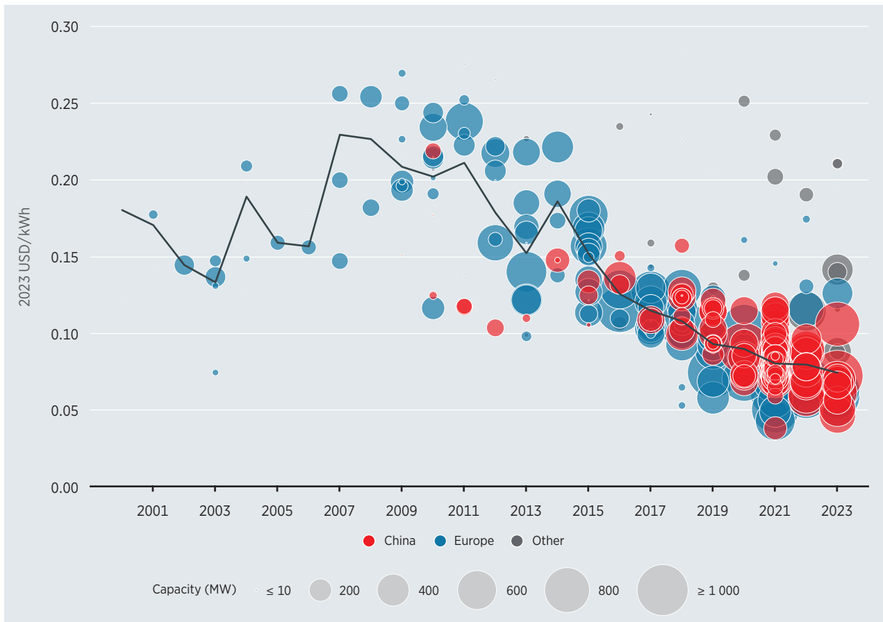
Figure 4.11 Offshore wind project and global weighted average LCOE, 2000-2023
