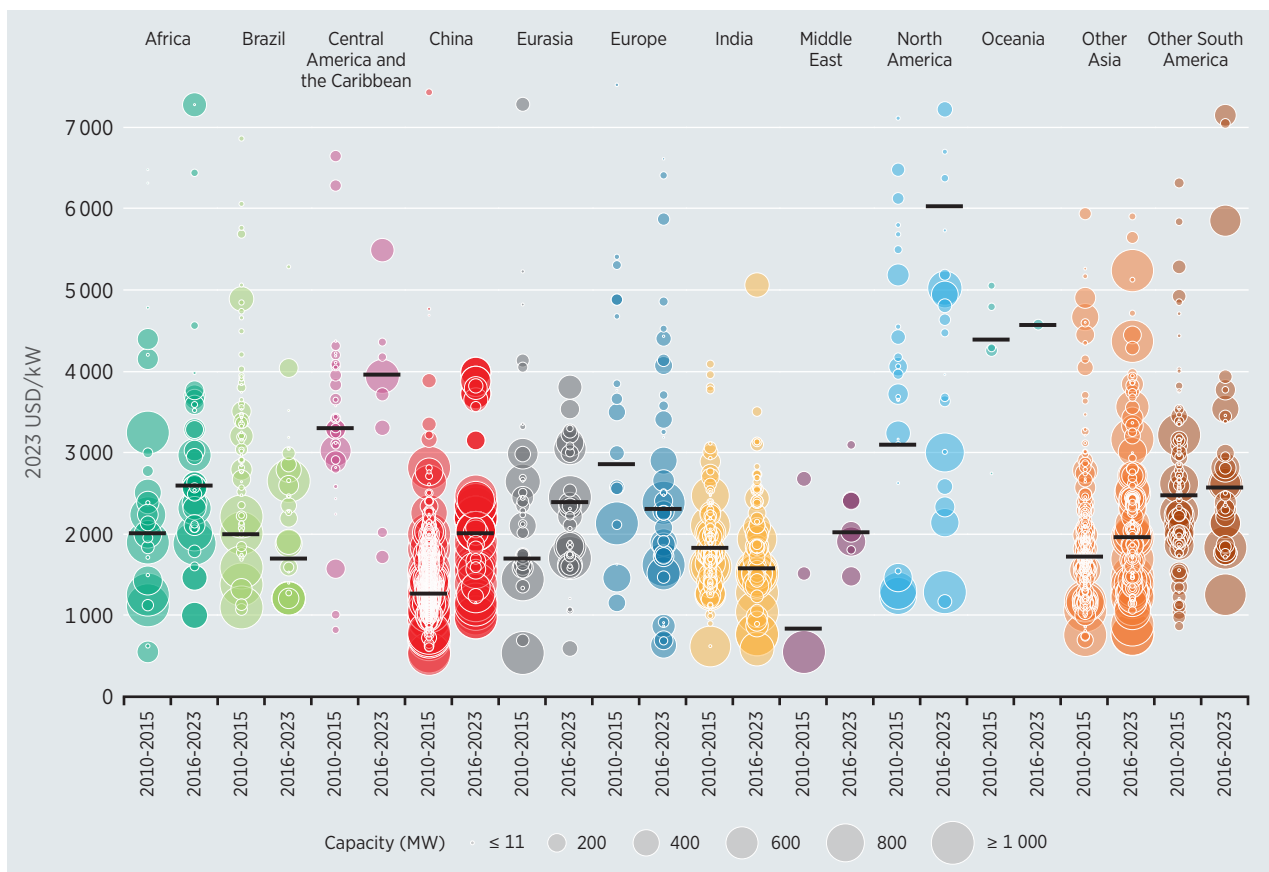
Figure 7.5 Total installed cost by project and capacity weighted averages for large hydropower projects by country/region, 2010-2023
